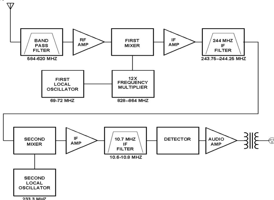
Fig 3 – Signal flow in a typical low-cost UHF wireless mic receiver
