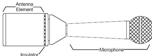
Fig 2 – A plug-on transmitter attached to a mic
