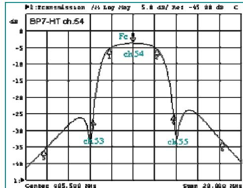
Fig 16 – This larger and more expensive multi-stage filter (about \$450) has both wider bandwidth and better rejection of adjacent transmitters. [The channel identification references CATV channels, not broadcast channels] These filters are from Tin Lee Electronics ([www.tinlee.com](http://www.tinlee.com))
