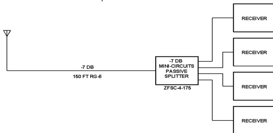
Fig 10 Moving the antenna closer to the talent puts 13 dB more signal at the antenna, but we lose 7 dB in the coax and 7 dB in a passive splitter for a net loss of 1 dB. But any TV interference (including overload or desense that it causes) is reduced by 14 dB!
