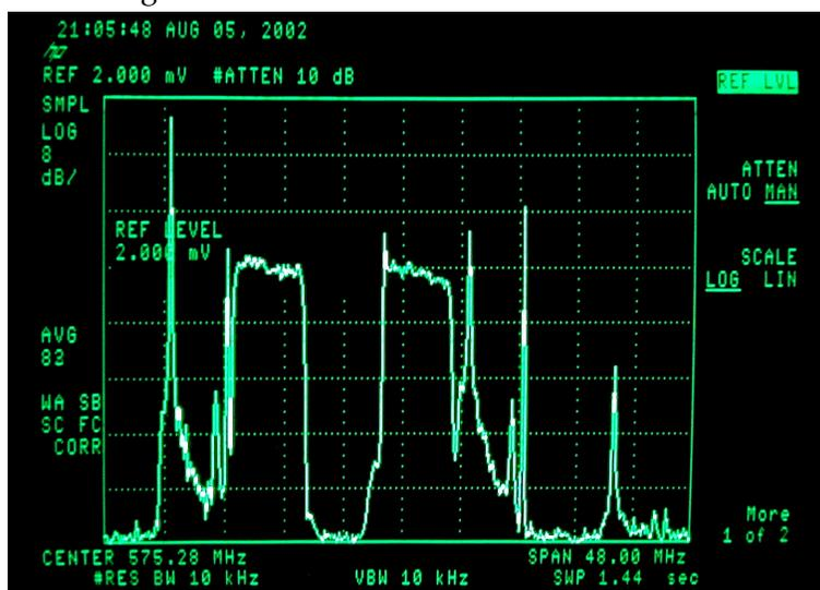
Fig 6. This spectrum analyzer's view of eight UHF TV channels clearly illustrates the nature of the interfering signals that a wireless mic system must compete with. Three analog TV stations and two DTV stations are transmitting in the eight TV channels shown in this scan. Five years ago, those digital transmitters weren't on the air!
