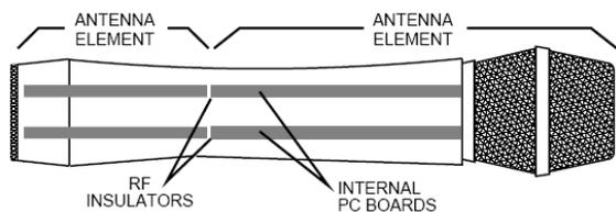
Fig 1 – A handheld transmitter
