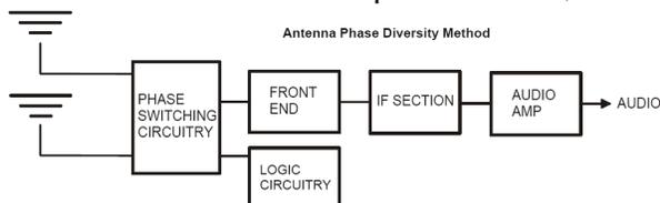
Fig 5c – Switched-antenna-polarity diversity
