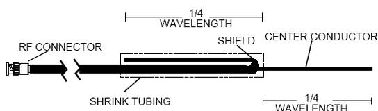
Fig 4a - This general purpose antenna is approximately omnidirectional
