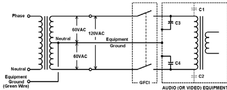
Fig 16 –A Balanced Power System per NEC 647 (2002)
