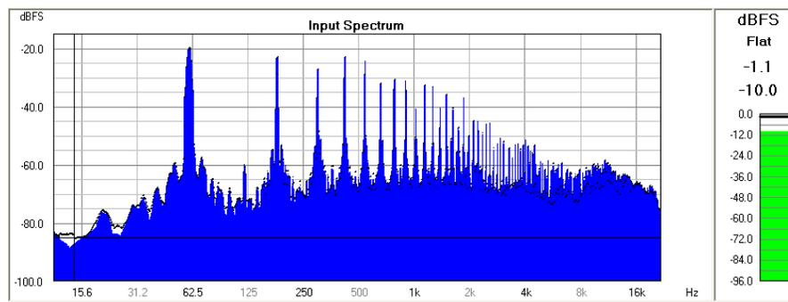
Fig 17 – Typical noise spectra on an equipment ground
