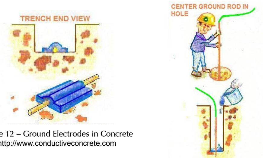
Figure 12 – Ground Electrodes in Concrete
