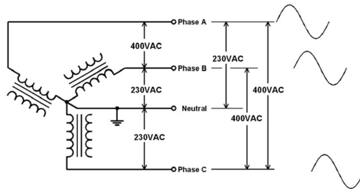
Figure 3b – Three Phase 400V/230V Power System
