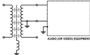
Figure 19c – Isolation Transformer showing inductance of earthing path
