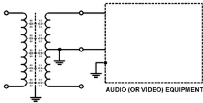
Figure 19b – An Isolation Transformer
