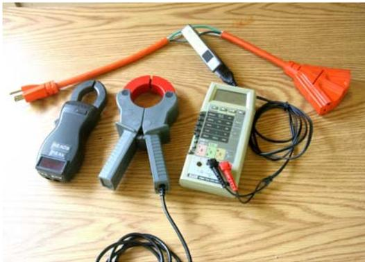
Fig 20 – Current probes and breakout cable
