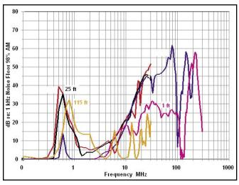
Fig 8 -- This mic had no problem with the AM broadcast transmitter, but it did receive interference from the ham transmitters and from some VHF TV.
