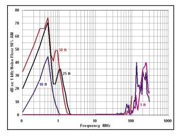
Fig. 4 – A mic with even greater susceptibility to AM broadcast RF
