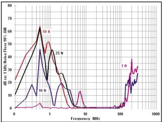
Fig. 3 – A mic with susceptibility to AM broadcast RF
