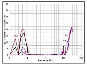
Fig. 7 – This mic has sufficient filtering to reject all but the strongest RF below 200 MHz. It experienced no interference from the AM broadcast or ham transmitters.
