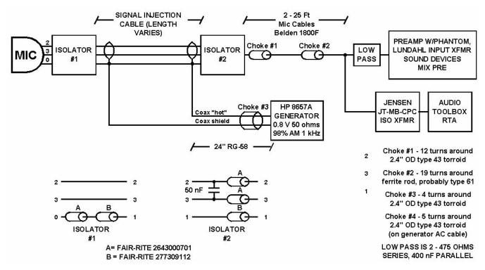
Fig 1-Test setup for susceptibility of microphones to RF on the signal pair.
