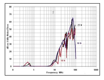
Fig. 2 – Differential mode susceptibility of a very good omni mic
