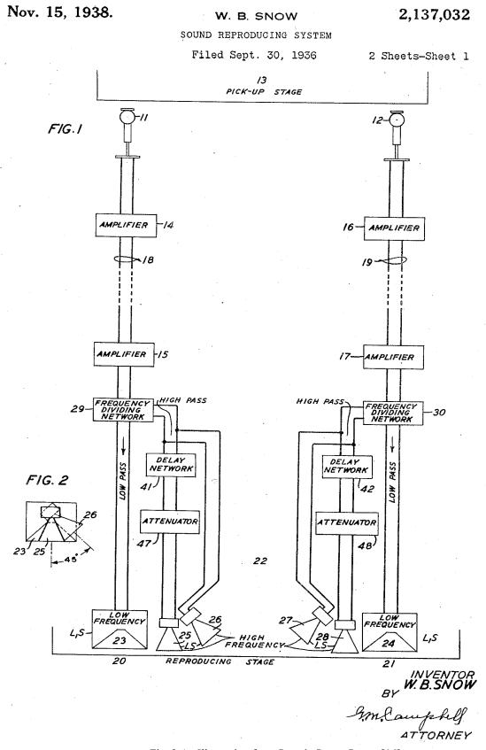
Fig. 2 An Illustration from Snow's Stereo Patent [16]
