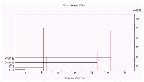
Fig 9 EASE prediction of direct sound arrivals at a seat near the left rear corner of the left center seating bank. A study of the results of calculations like this one is required for seats throughout the audience to verify that the design meets the criteria for good stereo.
