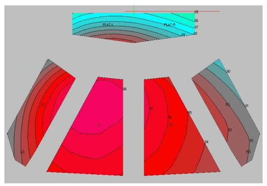
Fig 6. Predicted direct sound from a single  $90^{\circ}x$   $40^{\circ}$  loudspeaker, 9 m left of center, aimed to the center rear of the right center seating in the room of Figs. 4 and 5.
