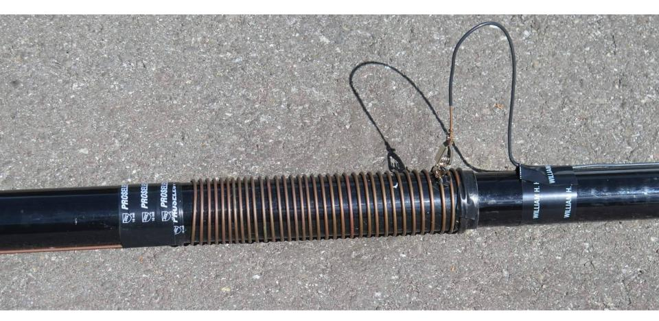
32 turns, #8 bare copper, tapped. Turns can be compressed or expanded for tuning
